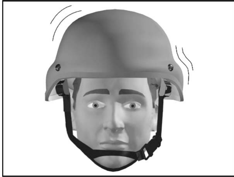
Figure 2-21. ACH too loose.
